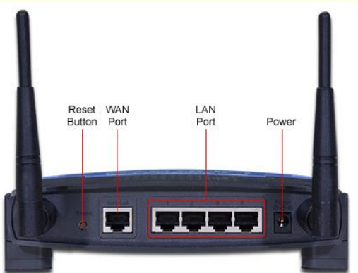
Hybrid Modem with WAN and LAN ports (necessary for Internet access) and wireless access
