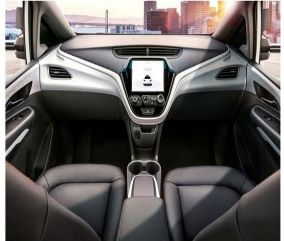
Welcome to the age of the truly driverless car: GM's latest self-driving vehicle is a modified Chevy Bolt without a steering wheel or pedals.
