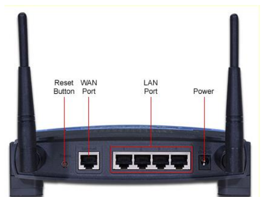
Hybrid Modem with WAN and LAN ports (necessary for Internet access) and wireless access
